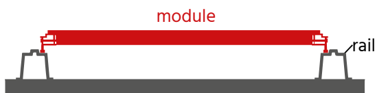
The rails guide the modules laterally.
